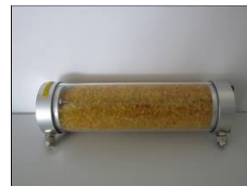
Dry Silica Gel in the DDU 570
