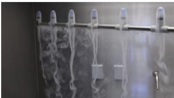
Discharge of the fog with the help of the CFG 291 distribution rake.
