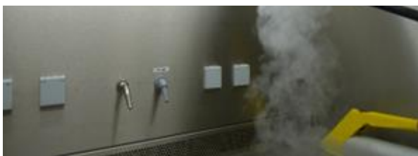
Discharge of the fog with the help of the one spot probe of CFG 291.
