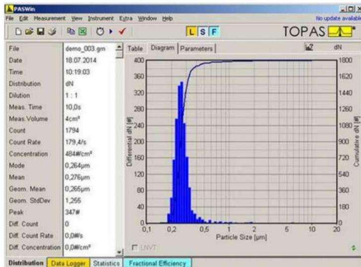
PASWin software for configuration, control, data logging and data analyses of particle counters and aerosol spectrometer
