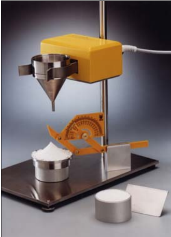
Determination of angle of repose with EMS 755
