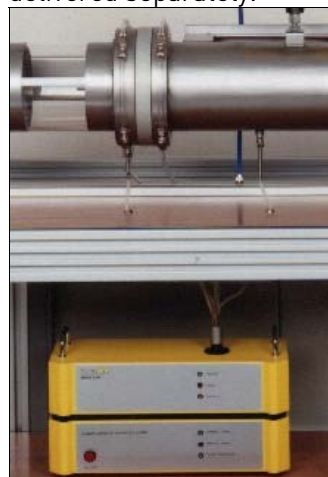
Effective measurement of particle size distributions with a laser aerosol particle size spectrometer LAP 322 (arrangement with sample switching unit below the test channel)
