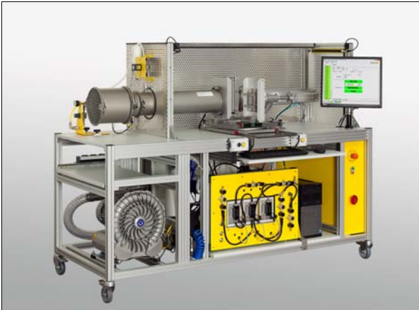
Filter test system AFC 132 / QC HEPA
